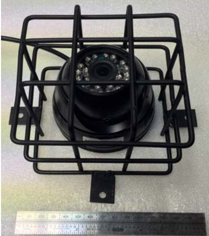
Steel Welded at all contact points
